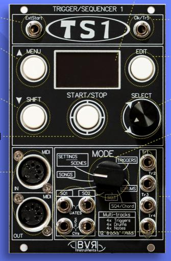
OLED screen with graphical user interface Displays current Mode.
